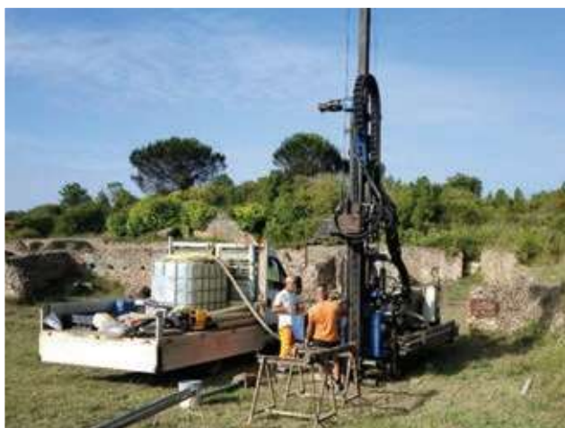
Port harbours, which offer a unique window into population, diet, health, technology, and environmental change, may also be traps for sedaDNA. The Ancient Ports of Europe: A Novel Genetic Window on Ancient Lives (PortGEN) project is using rigs to extract sediment cores from historic European and Mediterranean harbours, including Portus and Ostia – harbours that once served ancient Rome. © PortGEN
