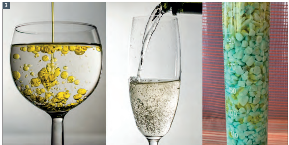
Figure 3: Imaging fluids in the subsurface using two glasses – one with olive oil and water (left) and one with sparkling wine and CO 2 (centre). On the right is a lab experiment showing olive oil (green) trapped as a residual phase in a granular water-saturated porous medium (scale in mm) as an analogue to CO 2 trapping in subsurface rock formations. Modified from Ringrose & Bentley (2021) Reservoir Model Design (2nd Ed.) Springer, Dordrecht. (Photos by Britta Paasch and Philip Ringrose.)
